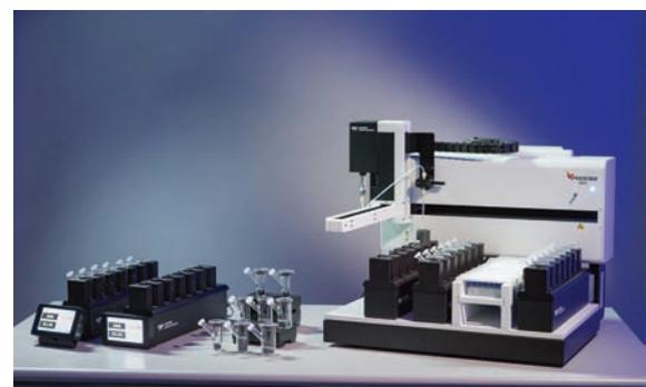
Figure 1. Phoenix DB-6 Manual Diffusion Systems (좌), Phoenix RDS Automated Diffusion Systems (우)
