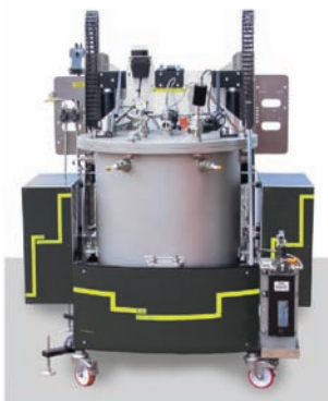
<BTC-500 / Large-scale, battery testing, adiabetic calorimeter>
