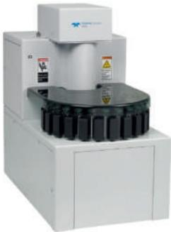
Versa Automated Headspace Vial Sampler
