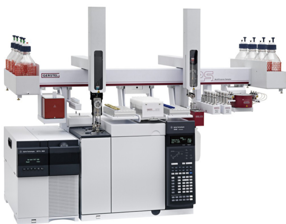
Figure 1: Instrument setup for the automated determination of THC and metabolites in blood serum. Dual Head MultiPurpose Sampler (MPS) equipped with agitator, standard wash station, trays for eluate vials, SPE cartridges and samples, SPE module, two solvent filling stations (SFS), Multi-Position evaporation station (mVAP) and solvent bottle station (from left to right). Left head with 10 µL syringe for injection, right head with 2.5 mL syringe for sample preparation steps. GC/MS system: Agilent GC 7890 / MSD 5977 (Agilent Technologies).
