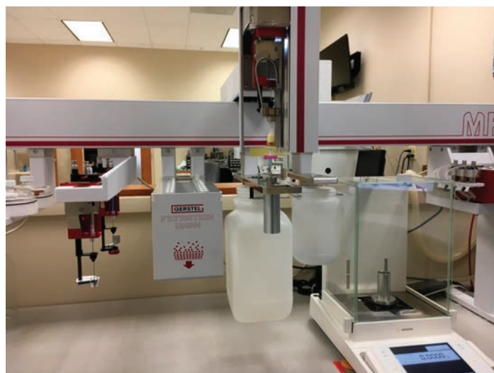
Figure 2: GERSTEL MPS roboticPRO sampler with GERSTEL DNPH Option.
