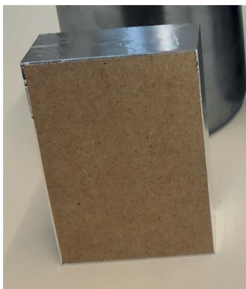
Figure 4: Medium-density fiber board (MDF) prepared in 6 cm x 9 cm size and all edges covered with aluminum foil. The sample was placed vertically in the DHS Large container.
