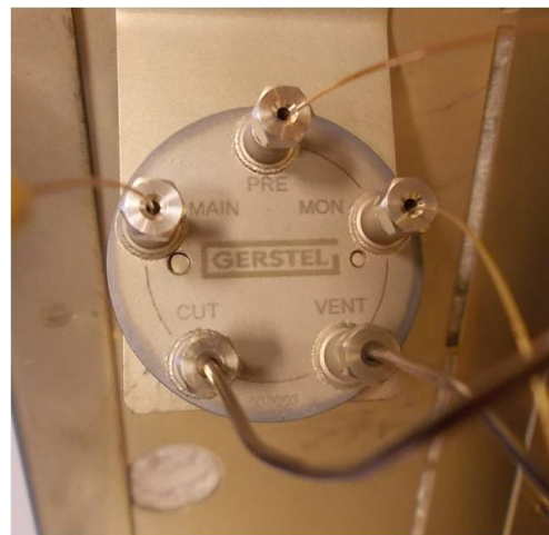
Figure 2: GERSTEL \mu\text{MCS} fraction distribution device.
