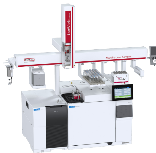
GERSTEL LabWorks Platform, here on an Agilent 8890 GC with 5977B MSD
