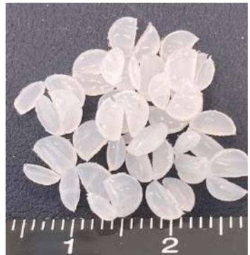
HDPE 0.48 g Pretreatment: Cut in half with nippers
