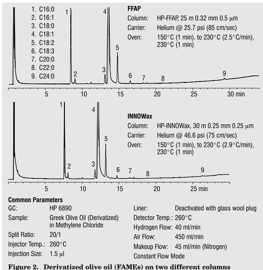
better peak symmetry than the Innowax column (a peak symmetry value of less than one indicates the peak is tailing). Similar results were obtained
