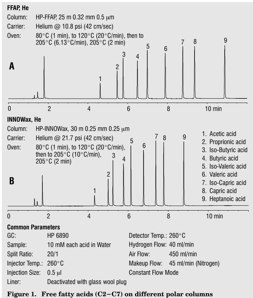
**Figure 1. Free fatty acids (C2–C7) on different polar columns**
